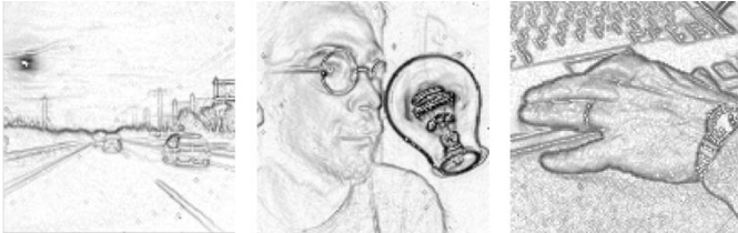
Fig. 14. Contrast representation with extreme inhomogeneities of illumination (left and center) and very weak contrasts (right).
