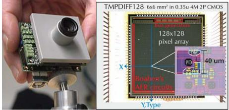
Each retina has  $128 \times 128$  pixels and the spike output addresses are captured by a computer and displayed for you. This chip is an Address-Event Representation (AER) chip. The pixels respond to movement, or more specifically, to *temporal contrast*. Each spike means that the log intensity has changed by a threshold amount *T* since the last event from that pixel.
