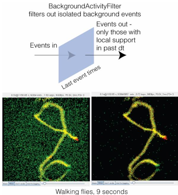
Fig. 3 Example of event-filtering. BackgroundActivityFilter filters out about 2/3 of the events that lack spatio temporal support, leaving only the walking fruit fly.
