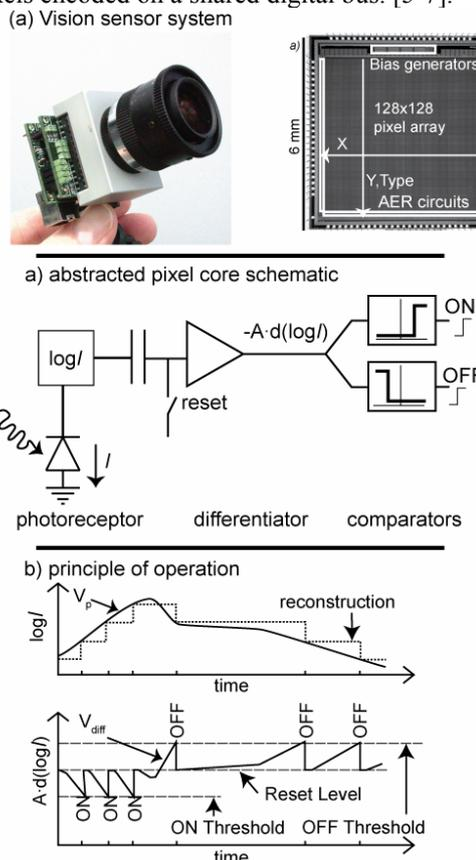
Fig. 1 DVS characteristics. a) the dynamic vision sensor with lens and USB2.0 interface; b) a die photograph labeled with components. Also shown is the row and column from a pixel that generates an event; c) abstracted schematic of the pixel which responds with events to fixed-size changes of log intensity; d) how the ON and OFF events are internally represented and output in response to an input signal.
