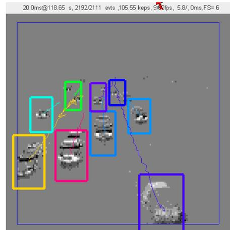
Fig. 5 Object tracking: RectangularClusterTracker tracks multiple cars from highway overpass.
