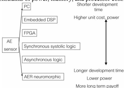
Fig. 6 Event processing hardware platforms. This paper described methods implemented mostly at the PC level, where development times are shortest.
