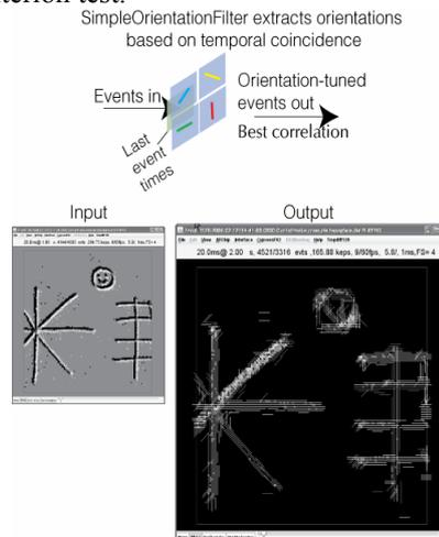
Fig. 4 Example of event labeler: SimpleOrientationFilter annotates events with the edge orientation. Each panel shows a different orientation type output.
