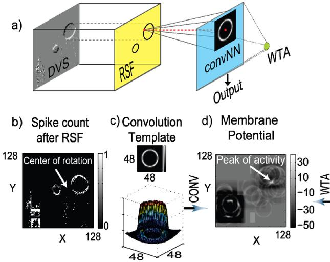
Figure 1. Network architecture (a) Architecture includes three stages: RSF, spiking convolution network (convNN), and WTA; (b-d) Example output from the architecture: (b) RSF output over 10ms, (c) convolution template (the top view and 3D view) and (d) instantaneous membrane potentials of convNN neurons.
