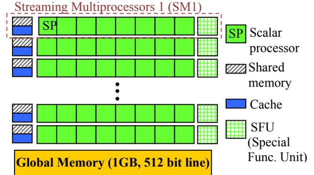
Figure 2. Simplified architectural view of CUDA GPU.
