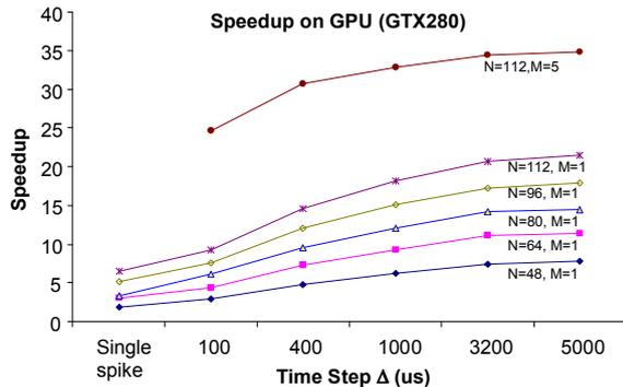
Figure 5. Kernel level speedup by running the application on NVIDIA GPU (GTX280).  $\Delta$  indicates the time step for grouping.  $N \times N$  gives the template size,  $M$  indicates the number of networks. Error bars are not plotted due to their insignificant variance.
