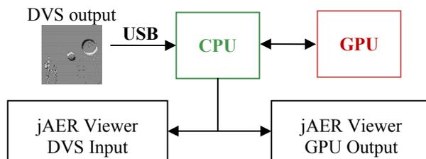
Figure 1: Demonstration setup. jAER [2] is used to interface with DVS chip and to visualize spikes.
