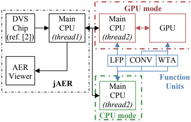
Figure 3. Experimental setup in CPU mode and GPU mode. jAER [10] is used to interface with AER DVS and to visualize AER spikes.
