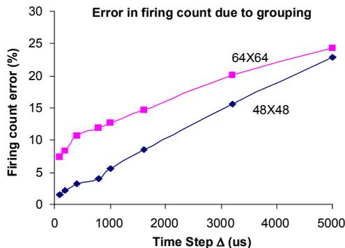
Figure 6. Error in the total firing count for different values of  $\Delta$  (time step) with template size 48x48 (in blue) and 64x64 (in magenta).
