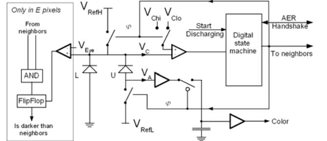
Fig. 3 Pixel architecture, including control state machine, sample and hold for the color value and the circuits for the computation of the eye feature (section C). The pixel consists of two photodiodes, two comparators, two source-followers, a capacitor and some digital control logic.
