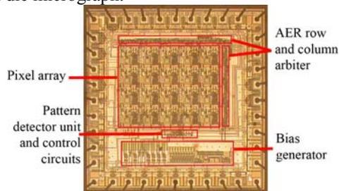
Fig. 4 Die micrograph. Die size is 2.2 by 2.2 mm.
