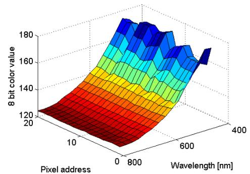
Fig. 6 Spectral response of all 20 pixels vs wavelength.
