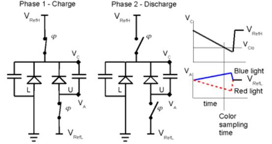
Fig. 2 The two phases of the pixel operation. Phase 1 recharges nodes  $V_C$  and  $V_A$  to reference values. In phase 2 both photodiodes are discharged by the photocurrents.  $V_A$  depends on the ratio of the photocurrents and therefore on the spectral content of the light.
