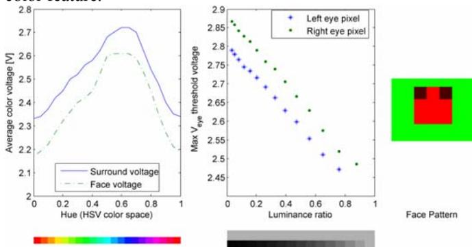
Fig. 8 Pattern detector circuit response. Left plot shows the output of the capacitive averaging circuits. Right plot shows the maximum  $V_{eye}$  threshold voltage at which the sensor still can detect an eye for the given luminance ratio between eye pixel and surround. Reference voltages are  $V_{chi}=2.985$  and  $V_{Cio}=2.463$  V. Right pattern is the stimulus “face” pattern.
