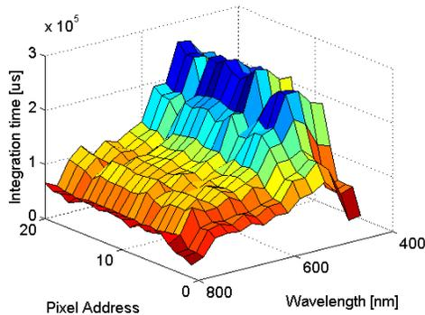
Fig. 7 Integration time for all 20 pixels vs wavelength. The integration time has been normalized by the irradiance measured with a Tektronix J17 photometer.
