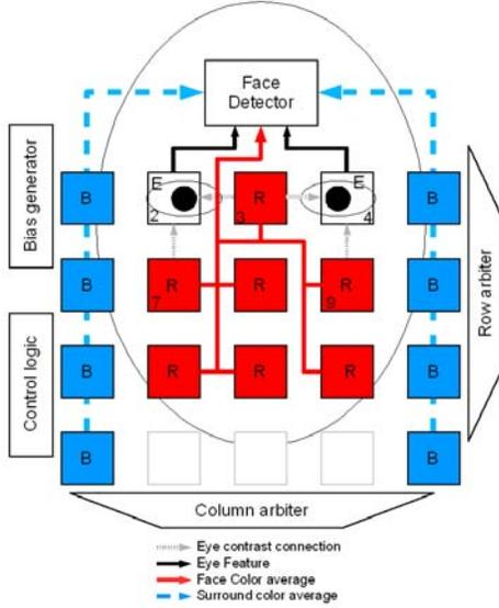
Fig. 1 Architecture of the face detector.
