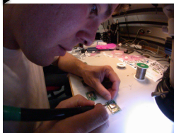
PCB SMD assembly
