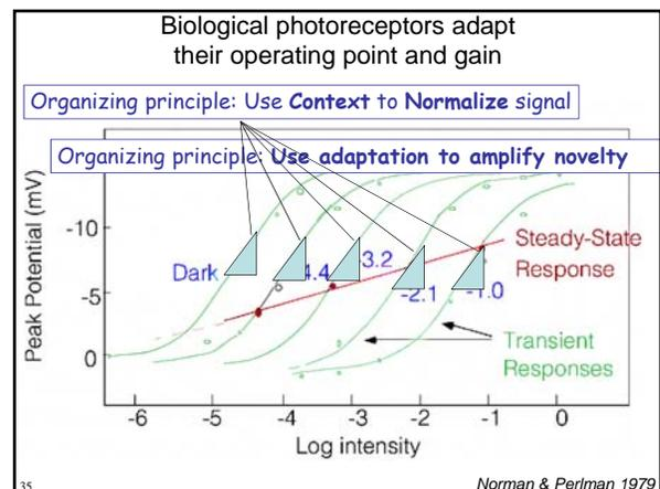
A logarithmic (or self-normalizing) representation of intensity is useful for representing object reflectance differences, rather than the illumination conditions.
