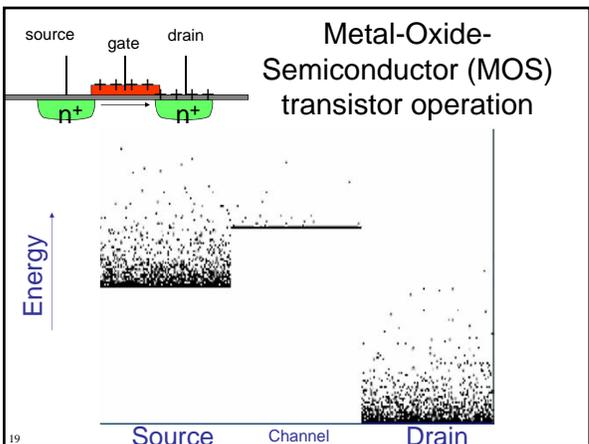
**Mechanism of *transconductance***
