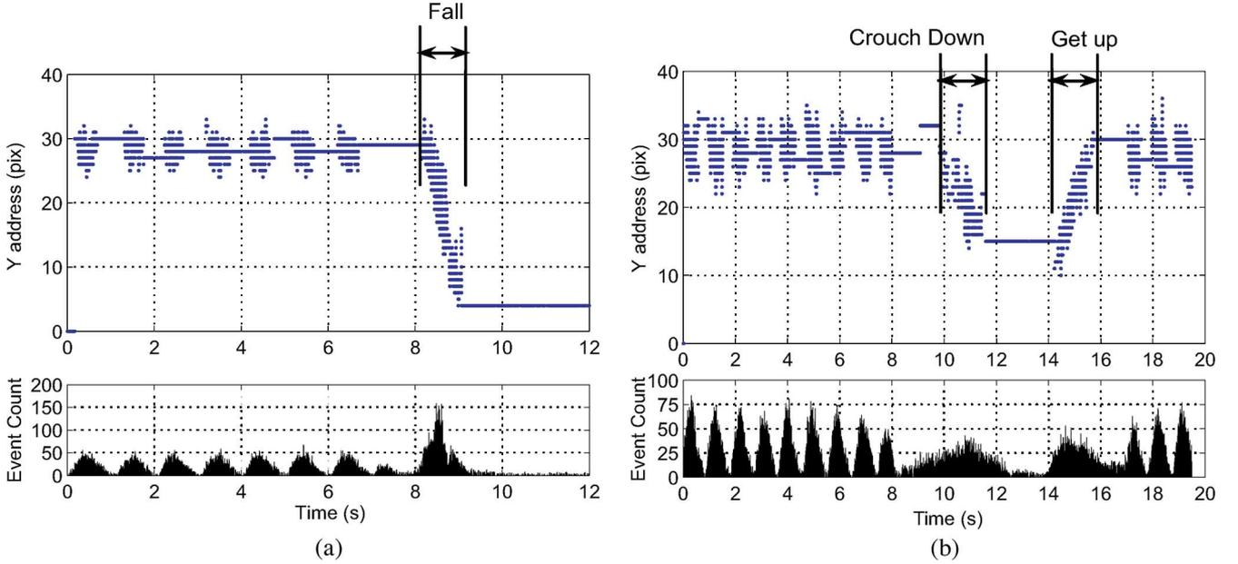
Fig. 7. Vertical address of the centroid events ( $Y_c$ ) (a) when a person falls, and (b) when a person crouches down. In (a), when the person falls, the centroid vertical address decreases by 25 pixels in 0.9 s. The event rate is approximately 5600 event/s. In (b), when the person crouches down, the centroid vertical address decreases by 20 pixels in 2 s. The event rate is approximately 310 event/s. The fall causes faster decrease in the vertical address than the crouch-down.
