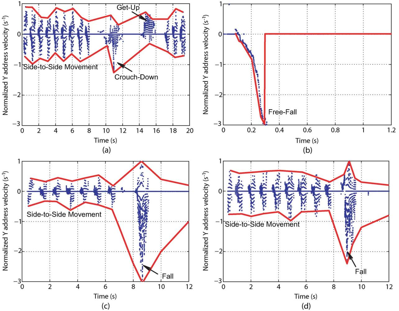
Fig. 8. Centroid vertical velocities ( $V_{y,norm}$ ) in address-event streams demonstrate the difference among four scenarios: (a) a person crouches down; (b) a box free-falls; (c) a person falls backward; and (d) a person falls forward. The velocities are normalized for distance between the imaged subject and the image sensor. The red lines in the figures outline the boundary of the peak vertical velocities.
