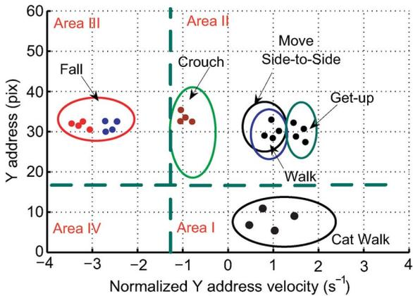
Fig. 9. Centroid address-event evaluation matrix of five common home-assisted living scenarios. The centroid vertical velocities are normalized for distance.
