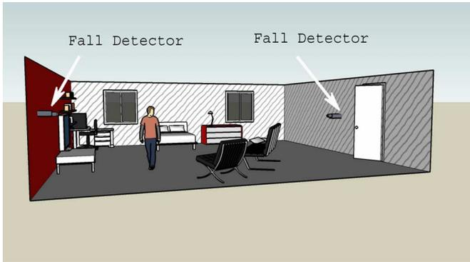
Fig. 1. Address-event fall detectors are used for assisted living applications. The detectors are mounted on the wall at a height of 0.8 m, which is approximately the same height of a light switch.
