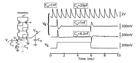
Fig. 9. Measurements of master bias stability.  $V_X$  is an external signal capacitively coupled into the  $V_R$  node.
