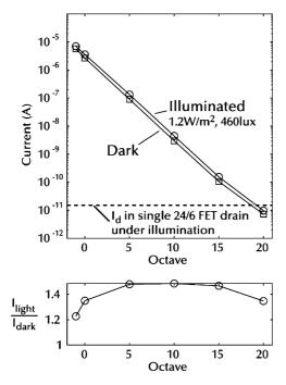
Fig. 14. Effect of illumination on generated currents.
