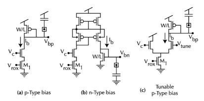
Fig. 5. Generating individual biases from the current splitter outputs.  $M_1$  has same W/L as  $M_{ro}$  in Fig. 1. The square attached to each capacitor represents a bonding pad.
