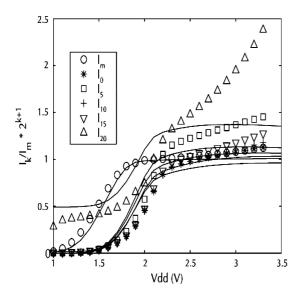
Fig. 17. Measured power supply sensitivity of the master bias current and splitter output currents.  $I_m = 1 \mu A$ , and each curve is normalized by its ideal value. The test transistor used to monitor the current was held at 0.3 V drain voltage, and  $R = 30 \text{ k}\Omega$  was used to make a master current of about 5  $\mu A$ .
