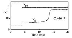
Fig. 10. Power control with  $V_{\rm pd}$  ( $V_{\rm pd}$  is rescaled). There was a 30-second delay since the last cycle. A high-impedance analog buffer was used to prevent a conductive path from  $V_{\rm n}$  to ground.
