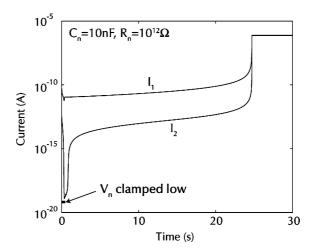
Fig. 3. Simulation of slow restart when off state is intentionally produced by clamping  $V_n$  low. A resistor  $R_n$  was connected between  $V_n$  and ground, and a large capacitance  $C_n = 10$  nF was used to demonstrate slow self-restart.
