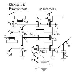
Fig. 4. Close-up of startup and power control circuits.
