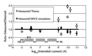
Fig. 15. Nonidealities of decade splitter built not using unit transistors. Points show ratio of measured current to ideal current and measured current to SPICE-simulation current for all instrumented splitter taps and individual biases. Error bars show variation over five chips. Inset shows current splitter transistor sizing.
