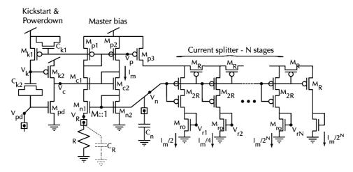
Fig. 1. Bias generator core circuits.  $I_m$  is the master current, and R is the external resistance. Transistor sizes are in units of  $\lambda$  (the scalable length parameter) and are listed in Table 1.  $C_{k1}$  and  $C_{k2}$  are MOS capacitors.  $M_R$  and  $M_{2R}$  are identically sized unit transistors. The squares represent bonding pads and recommended external connections.
