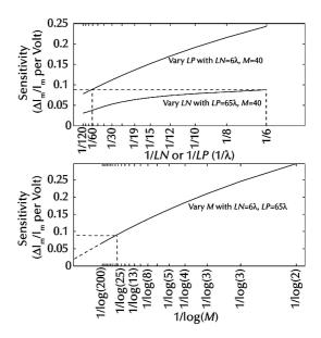
Fig. 24. Scaling of power supply sensitivity of the low-voltage version of the master bias current with circuit parameters. The dashed lines indicate default values, with LN =  $6 \lambda$ , LP =  $65 \lambda$ , and M = 40.
