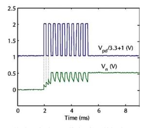
Fig. 11. Restarting the master bias by using multiple pulses on  $V_{\rm pd}$  when there is a conductive path from  $V_{\rm n}$  to ground.
