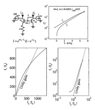
Fig. 2. Detailed action of degenerated mirror showing entire range of operating currents, from "off" to intended currents. Current is normalized to the  $M_{n2}$  off-current, and voltages are in units of  $U_T$ . R is in units  $U_T/I_0$ . Bottom left shows the currents on a linear scale whereas bottom right shows them on a log scale.
