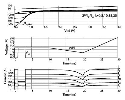
Fig. 23. Simulation results for a master bias and 20-stage current splitter from a 0.18  $\mu$  1.8 V process. The top traces are from a DC sweep of the power supply voltage and the lower traces show a transient simulation where  $V_{dd}$  and power control  $V_{pd}$  were both varied.
