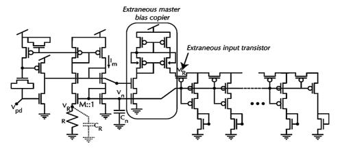
Fig. 7. Measured bias generator circuit.
