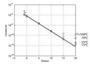
Fig. 19. Temperature measurements of bias generator core circuit. Plot shows master bias and splitter behavior at four temperatures. The straight lines show theoretical  $I_m/2^{\text{(Octave+1)}}$  predictions of the current.
