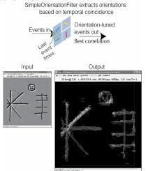
Fig. 4 Example of event labeler: SimpleOrientationFilter annotates events with the edge orientation. Each panel shows a different orientation type output.
