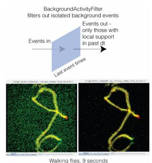
Fig. 3 Example of event-filtering. BackgroundActivityFilter filters out about 2/3 of the events that lack spatio temporal support, leaving only the walking fruit fly.
