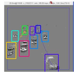
Fig. 5 Object tracking: RectangularClusterTracker tracks multiple cars from highway overpass.
