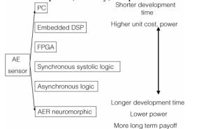
Fig. 6 Event processing hardware platforms. This paper described methods implemented mostly at the PC level, where development times are shortest.
