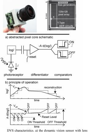
Fig. 1 DVS characteristics. a) the dynamic vision sensor with lens and USB2.0 interface; b) a die photograph labeled with components. Also shown is the row and column from a pixel that generates an event; c) abstracted schematic of the pixel which responds with events to fixed-size changes of log intensity; d) how the ON and OFF events are internally represented and output in response to an input signal.
