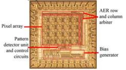
Fig. 4 Die micrograph. Die size is 2.2 by 2.2 mm.
