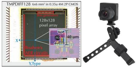
Each retina has 128x128 pixels and the spike output addresses are captured by a computer and displayed for you in the jAER software. This chip is an Address-Event Representation (AER) chip which means that the output of the camera is a stream of time-stamped address-events, which are active pixel addresses. The pixels respond to
