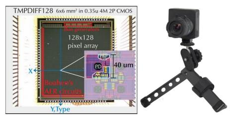
Each retina has 128x128 pixels and the spike output addresses are captured by a computer and displayed for you in the jAER software. This chip is an Address-Event Representation (AER) chip which means that the output of the camera is a stream of time-stamped address-events, which are active pixel addresses. The pixels respond to
