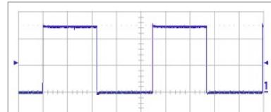
Fig. 2: Execution time of the analogRead function.
