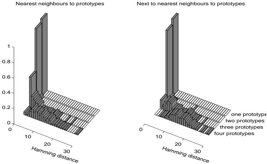
Figure 4: The distribution of Hamming distances of target attractors for stimuli in a sphere (left: Hamming radius 1, right: Hamming radius 2) surrounding the prototypes in state space, for networks with p learnt prototypes.
