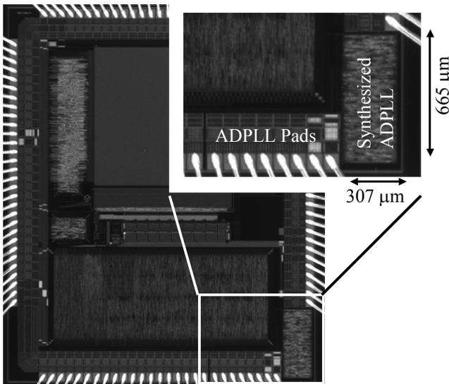
Figure 9. Chip microphotograph of the 0.35  $\mu\text{m}$  PLL (lower right corner) realized as part of a preprocessing pixel sensor SOC (backdrop)
