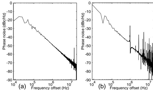
Figure 7. Phase noise (dBc/Hz) of DCO chain at fixed length corresponding to 91MHz (a) and PLL mode at 85 MHz with a reference clock frequency of 10 MHz
