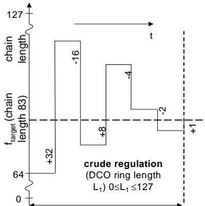
Figure 3. Frequency acquisition and control scheme of the ring length tuning.
