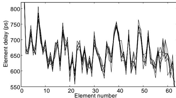
Figure 8. Delay of DCO elements in chain, measurement curves for several 0.35  $\mu\text{m}$  ICs overlaid.
