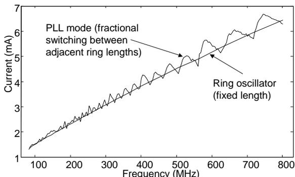
Figure 6. Current consumption as function of frequency for 0.13  $\mu\text{m}$  PLL
