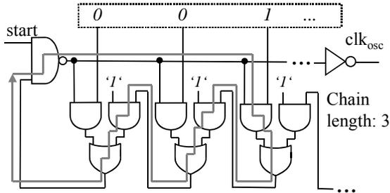
Figure 2. Oscillator chain for a one-hot coded length of three
