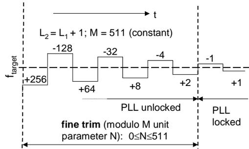
Figure 4. Frequency acquisition and control scheme of DCO
