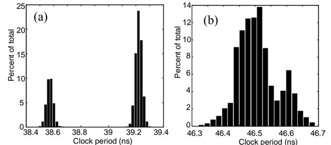
Figure 5. Histogram of sample clock periods for (a) 0.35  $\mu\text{m}$  PLL and (b) 0.13  $\mu\text{m}$  PLL.
