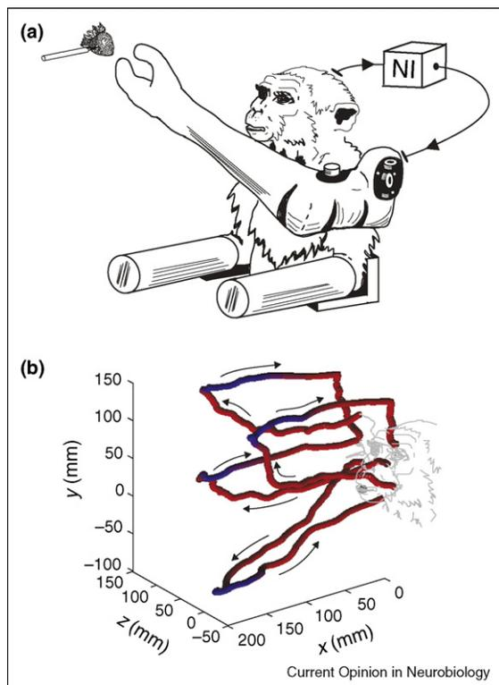
Cortical control of a prosthetic arm for self-feeding. **A.** Setup with hand-restrained monkey controlling a prosthetic arm using a neural interface (NI). Food targets were presented randomly in space that the animal could grasp, bring to the mouth, and eat. **B.** Spatial trajectory of robotic endpoint position of four consecutive trials. Color indicates gripper aperture (red: open, blue: closed). Modified with permission from [26\*\*].
