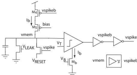
Fig. 2. The soma circuit implements an integrate-and-fire model.
