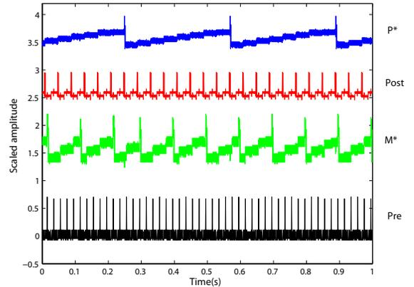
Fig. 3. Timing diagram of  $M^*$  and  $P^*$  at a learning synapse receiving a regular 50 Hz input spike train (pre) and a postsynaptic rate of 25 Hz (post).  $P(t)$  is sampled by every postsynaptic spike onto  $P^*(t)$  and  $M(t)$  is sampled by every presynaptic spike onto  $M^*(t)$ . Curves are offset from one another for ease of visibility.
