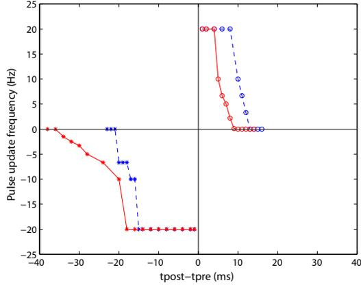
Fig. 4. Frequency of tunneling and injection pulses for a presynaptic input rate of 20 Hz and a postsynaptic rate of 20 Hz. The curves are obtained with various values of  $\tau_+$  and  $\tau_-$ .
