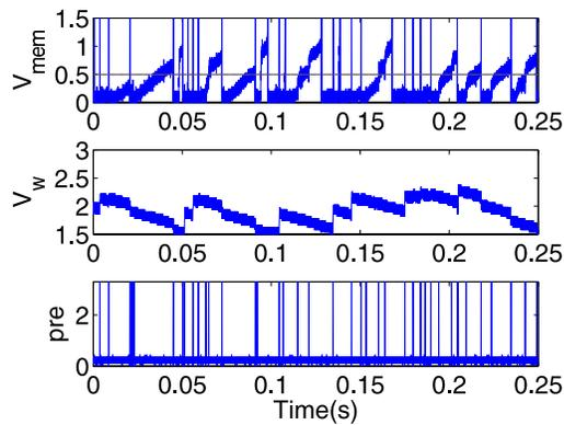
Fig. 3. Synaptic weight updates. Depending on the state of  $V_{mem}$ , the weight  $V_w$  is either increased or decreased with every pre-synaptic spike. Simultaneously, the bi-stability circuit drives  $V_w$  to the synapse's low stable state as long as  $V_w < V_{wth}$  ( $V_{wth} = 2.5V$  in this example).
