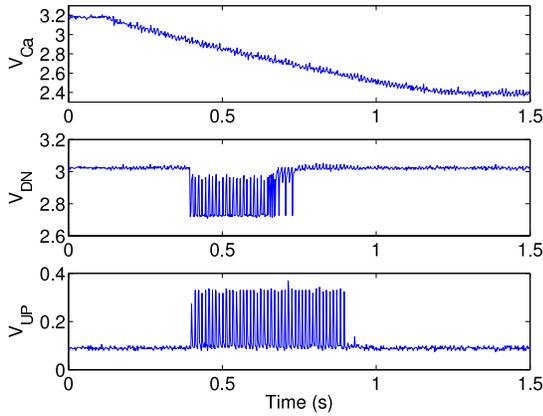
Fig. 2. Post-synaptic circuit data. (a) State of the  $V_{UP}$  and  $V_{DN}$  voltages are active only if the  $V_{Ca}$  signal is in an intermediate range.
