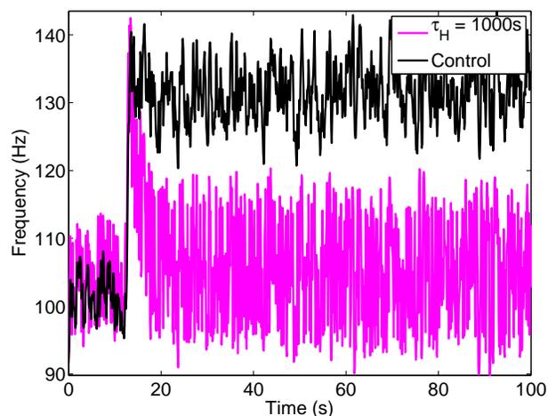
Figure 6. Homeostatic control adding high frequency fluctuations to the injection current: we replicate the same experiment of Fig. 5, adding random noise, for the time constant  $\tau_H = 1000s$ ; the black line shows the output of the neuron for a step in the input current level when the homeostatic control is not enabled. The blue curve shows how the DC offset in the firing rate is corrected, without affecting the high frequencies.
