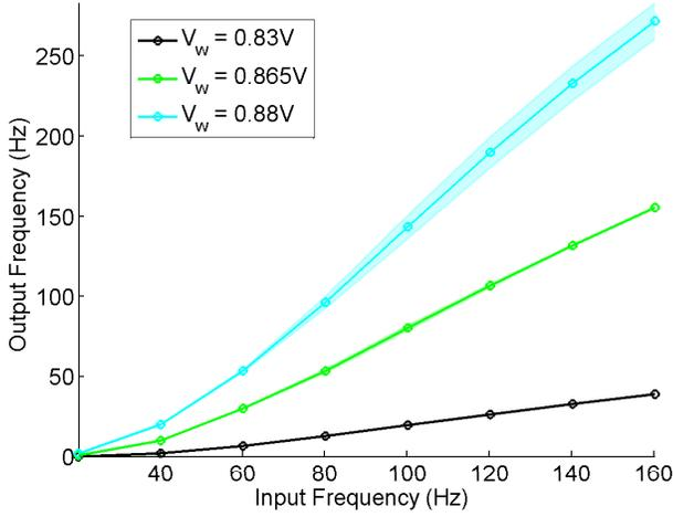
Figure 3. Firing rates mean and standard deviation (over 10 repetitions of the same experiment) of the I&F neuron when its input synapse is stimulated with regular spike trains, for different values of  $V_w$ . The measures are consistent with our mathematical analysis: the output frequency is linear with the mean current injected by the synapse (Eq. 8), the current is in turn linear with the synaptic input frequency (Eq. 7).
