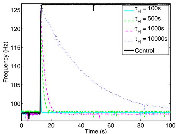
Figure 5. Homeostatic response to a step-wise DC shift in the neuron's instantaneous firing rate. The thick black line shows the output of the neuron for a step in the input current level when the homeostatic control is not enabled. The other curves show how the firing rate goes back to the initial activity level for different time constant of the homeostatic control.
