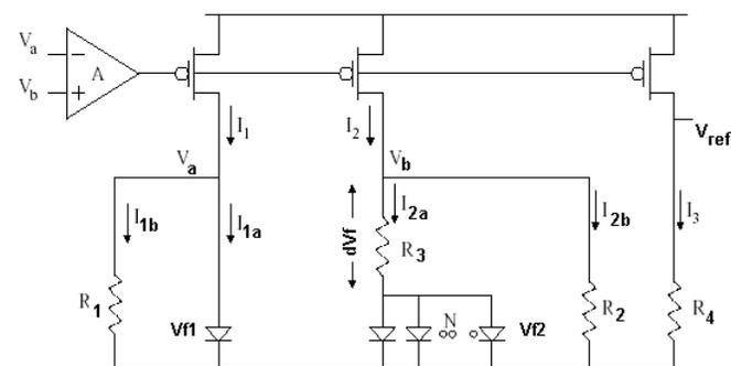
Fig. 6. Simplified schematic of the bandgap reference generator circuit. In practice  $R_1$  and  $R_2$  were made of two series resistors each, such that portion of  $V_a$  and  $V_b$  were feedback to the amplifier input.
