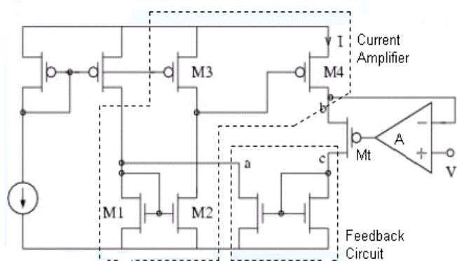
Fig. 5. Schematic of the circuit for testing the tail current source. M4 is the current source; Mt and amplifier A are used to fix the node voltage b externally.
