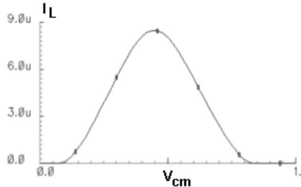
Fig. 4. Simulated output shows the required shape for the non-linear level shift current,  $I_L$ .
