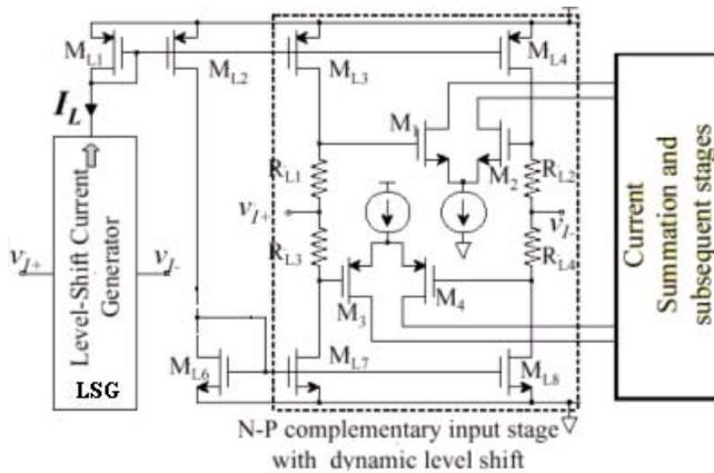
Fig. 3. The level shift current  $I_L$  driven through  $R_{L1-4}$  to generate input common mode voltages for n- and p-pair.
