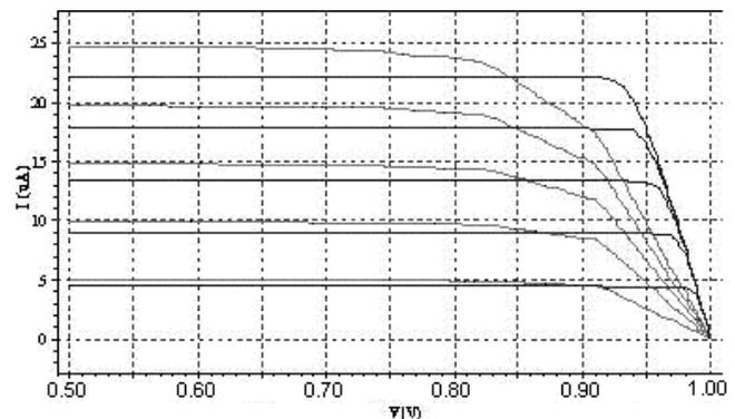
Fig. 8. Output impedance and  $V_{compliance}$ , tested for the tailcurrent source and a conventional cascoded current source.
