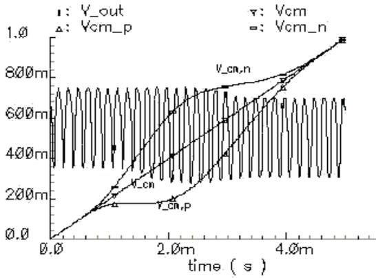
Fig. 9. Input common mode of the amplifier varied along with a very small differential voltage superimposed on it. The figure shows the open loop gain at different common mode voltage.
