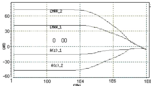
Fig. 10. The increase in CMRR in high impedance tail current source (CMRR\_2) is due to the decrease in common mode gain A(c)\_2.
