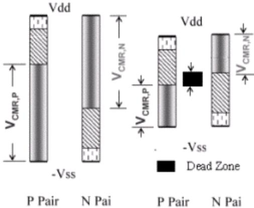
Fig. 2. The figure shows the available common-mode voltage for n- and p-differential pair.
