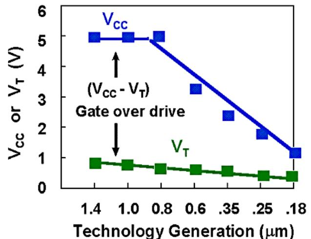
Fig. 1. Trend of supply voltage ( $V_{CC}$ ) and threshold voltage ( $V_T$ ) reduction with changing technology [2]. This shows the limitation in overdrive voltage available for analog design.
