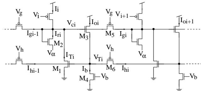
**Fig. 1.** Circuitry showing coupling between two excitatory neurons in an array of  $N$  excitatory neurons (in this paper,  $N=20$ ). The inhibitory circuit is local to each pixel. The circuit in each excitatory neuron consists of an input current source,  $I_i$ , and transistors,  $M_1$  to  $M_3$ . The inhibitory transistor is a fixed current source,  $I_b$  through  $M_4$ . The input to the inhibitory transistor,  $I_{oi}$  is normalized with respect to  $NI_b$ .
