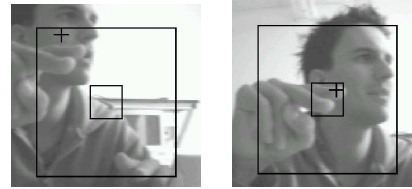
Figure 6: Sensor view just before the movement command (left image): the focus of attention has just switched to the top left corner. Sensor view just after the camera movement (right image): the focus of attention is now centered with the salient stimulus.
