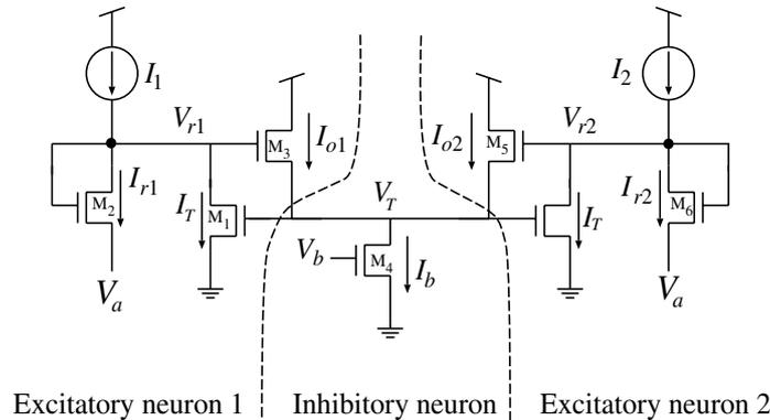
Fig. 2. Circuitry for two excitatory neurons and the global inhibition neuron,  $M_4$ . The circuit in each excitatory neuron consists of an input current source,  $I_1$ , and transistors,  $M_1$  to  $M_3$ . The inhibitory transistor is a source of a fixed current,  $I_b$ . The output currents  $I_{o1}$  and  $I_{o2}$  are normalized with respect to  $I_b$ . The width and length of all transistors in the excitatory neuron circuit are  $7.2 \mu\text{m}$ .
