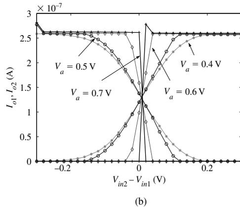
Fig. 4. Response of two neurons in the network shown in Fig. 2. The parameter  $V_a$  determines whether the network operates in the soft-max regime or the WTA regime. (a) Output currents  $I_{o1}$  and  $I_{o2}$  as functions of  $V_a$  for a subthreshold bias current and  $V_{in} = 4.0$  V to 4.3 V. (b) Output currents as functions of the differential input voltage,  $V_{in2} - V_{in1}$ , with  $V_{in1} = 4.3$  V.
