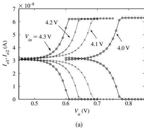
Because  $V_T$  depends on the input current,  $V_a$  increases for decreasing  $V_{in}$  (increasing input current).
