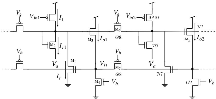
Fig. 3. Network of 20 excitatory neurons that are coupled together by diffusers or pseudoconductances ( $M_6$  and  $M_7$ ). The inhibitory transistor,  $M_1$ , is local to each neuron. The sizes of the transistors are in units of micrometers. This circuit was fabricated in a 2  $\mu\text{m}$  CMOS technology.
