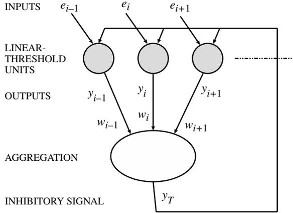
Fig. 1. Architecture of a recurrent network which consists of  $N$  linear threshold excitatory neurons (shaded circles) and one global inhibitory neuron (open ellipse). The inputs to the excitatory neurons are described by  $e$ . The global inhibitory signal,  $y_T$ , to the excitatory neurons, depends on the weights,  $w$ , and output states,  $y$ , of the neurons.
