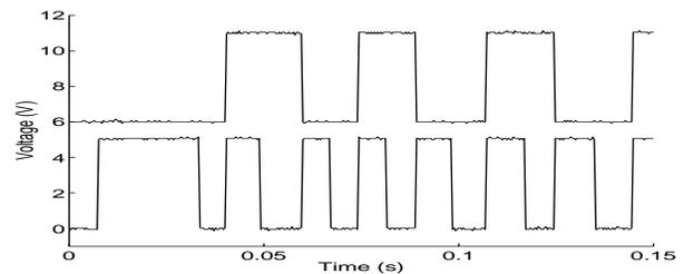
**Fig. 4.** Output of least significant bit (bottom trace) and second-least significant bit (top trace, displaced by 6V) of the 'X' address in response to a target moving from right to left.
