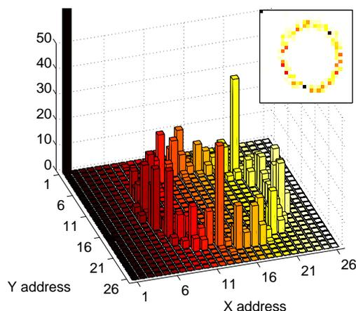
**Fig. 5.** Histogram of the addresses measured from the sensor's address encoders in response to a target moving on a circular trajectory.
