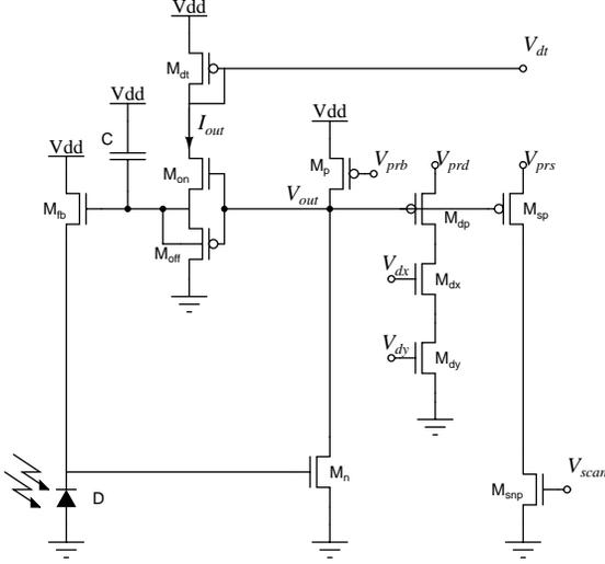
Fig. 1. Differentiating adaptive photoreceptor circuit.
