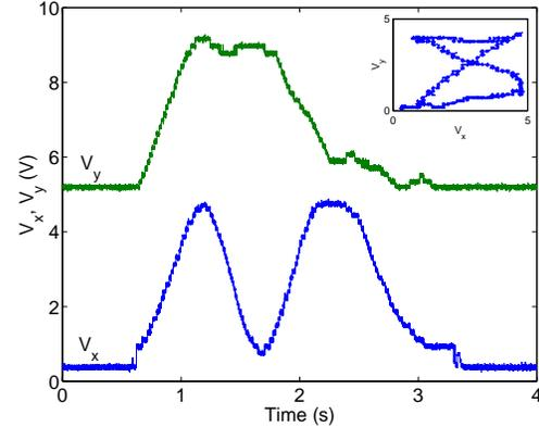
**Fig. 3.** Output of the analog P2V circuits in response to a target moving from the bottom left corner to the top right one, on to the top left, to the bottom right, and back to the bottom left corner.
