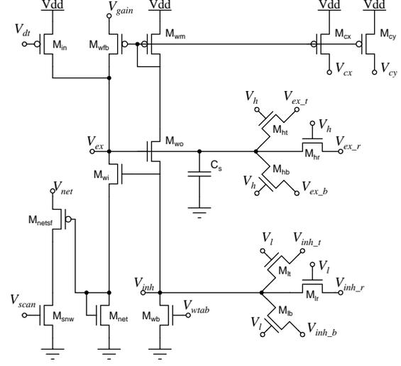
Fig. 2. Hysteretic WTA circuit with spatial coupling.
