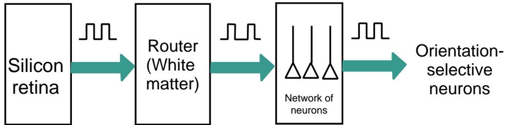
Figure 1: Block diagram of a multi-chip system in which virtual connections from a set of neurons on a silicon retina onto another set of neurons on a transceiver chip are described using the router module. The router communicates with the multi-neuron chip if the spike address from the retina falls within the lookup table programmed on this module.
