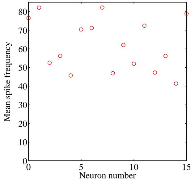
Figure 2: Distribution of the mean spike rates of the 16 neurons on the multi-neuron chip for a regular input spike train of 50 Hz. Due to circuit mismatches, the steady-state spike rate varies among the neurons.
