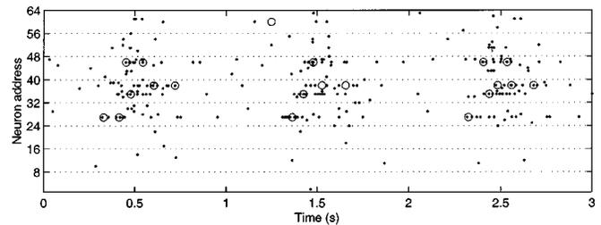
Fig. 8. Raster plot of the activity of the neurons of both transient imager chip (dots) and selective-attention chip (circles) in response to the flashing LEDs. To plot the data from both chips using an address space with the same resolution, we subsampled the addresses of the transient imager chip. The LEDs flashed approximately at 0.25, 1.25, and 2.25 s.
