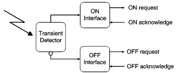
Fig. 4. Block diagram of irradiance transient detector with event-based communication interface.
