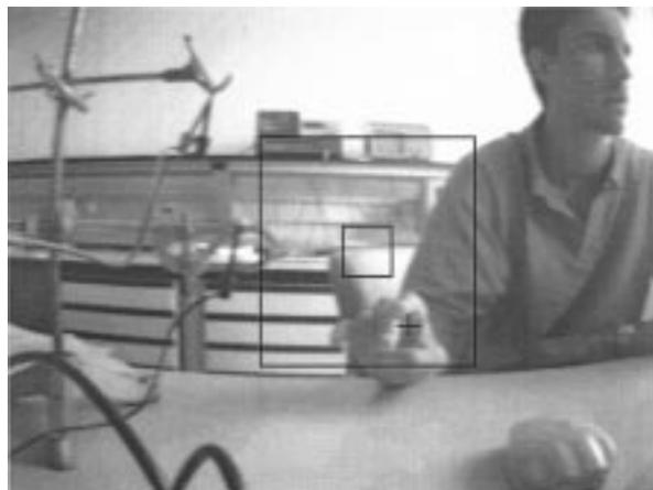
Fig. 6. Image captured from the CCD camera mounted next to the transient imager. The outer frame shown in the image corresponds to the field of view of the transient imager, whereas the inner frame is drawn to evidence the transient imager's central region. The cross to the bottom right of the image center represents the location of the focus of attention currently computed by the selective-attention chip.
