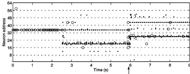
Fig. 10. Raster plot of the activity of the neurons of the transient imager chip (dots) and of the selective-attention chip (circles) in response to two flashing LEDs. The focus of attention shifts from a central region of the imaging array to a peripheral one (see circles at  $2 \text{ s} \leq t < 6 \text{ s}$ ). Consequently, the system makes a camera movement, at the time indicated by the vertical arrow, and re-centers the attended location.
