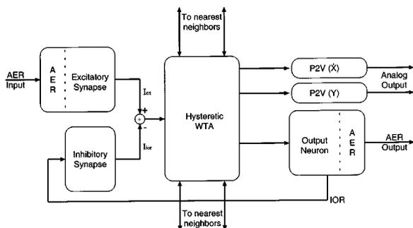
Fig. 5. Block diagram of a basic cell of the  $8 \times 8$  selective-attention architecture.
