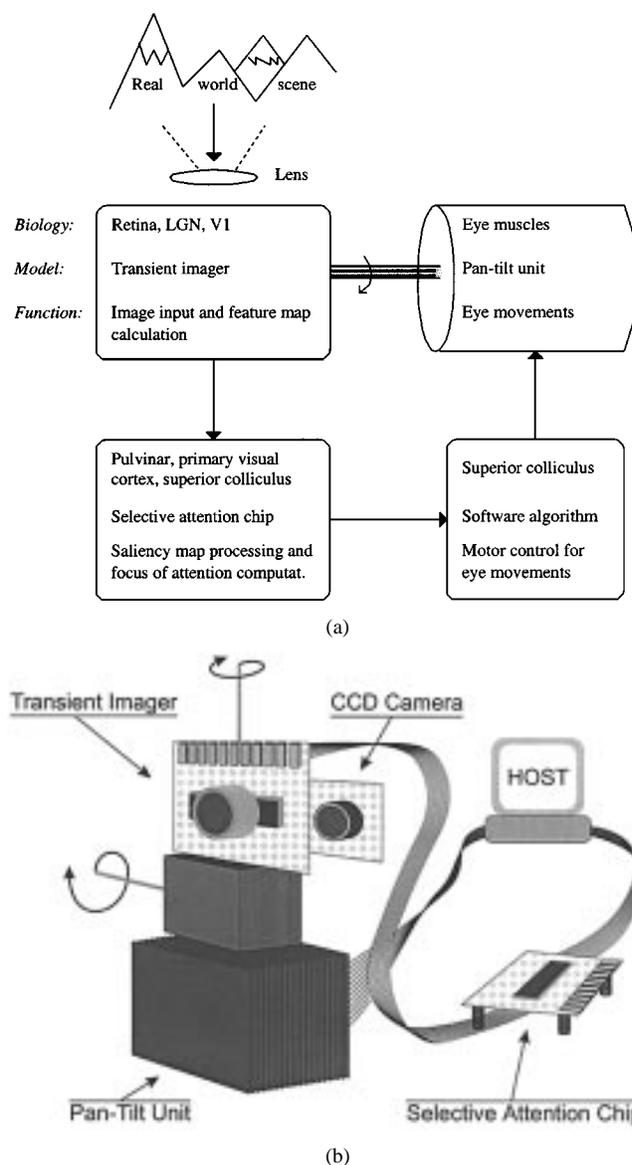
Fig. 2. (a) Block diagram of the sensory-motor selective-attention model. The figure shows the basic computational blocks used, as well as the corresponding biological analogs and their function. (b) Schematic diagram of the active-vision setup. The neuromorphic imager, mounted on a pan-tilt unit, transmits its output to the selective-attention chip. The latter sends the results of its computations to a host computer which uses this data to drive the pan-tilt unit’s motors.
