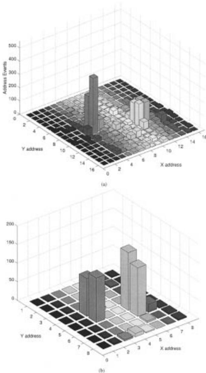
Fig. 7. (a) Histogram of events generated by the transient imager pixels in response to two diffused flashing LEDs. The LED stimulating the region around pixel (5,9) has higher contrast than the other LED. (b) Histogram of events generated by the selective-attention chip in response to the events generated by the transient imager chip.
