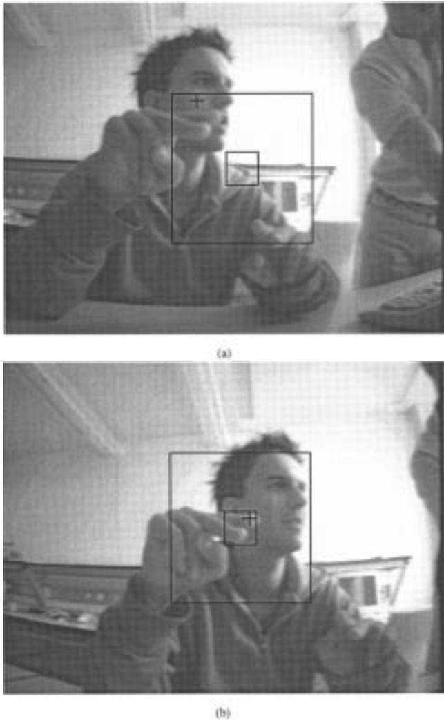
Fig. 12. Saccadic eye movements in response to moving fingers. (a) CCD camera snapshot taken before the saccadic eye movement (the focus of attention has just switched from one hand to the other). (b) CCD camera snapshot taken just after the saccadic eye movement (the focus of attention and the salient stimulus are now in the center of the imaging array).
