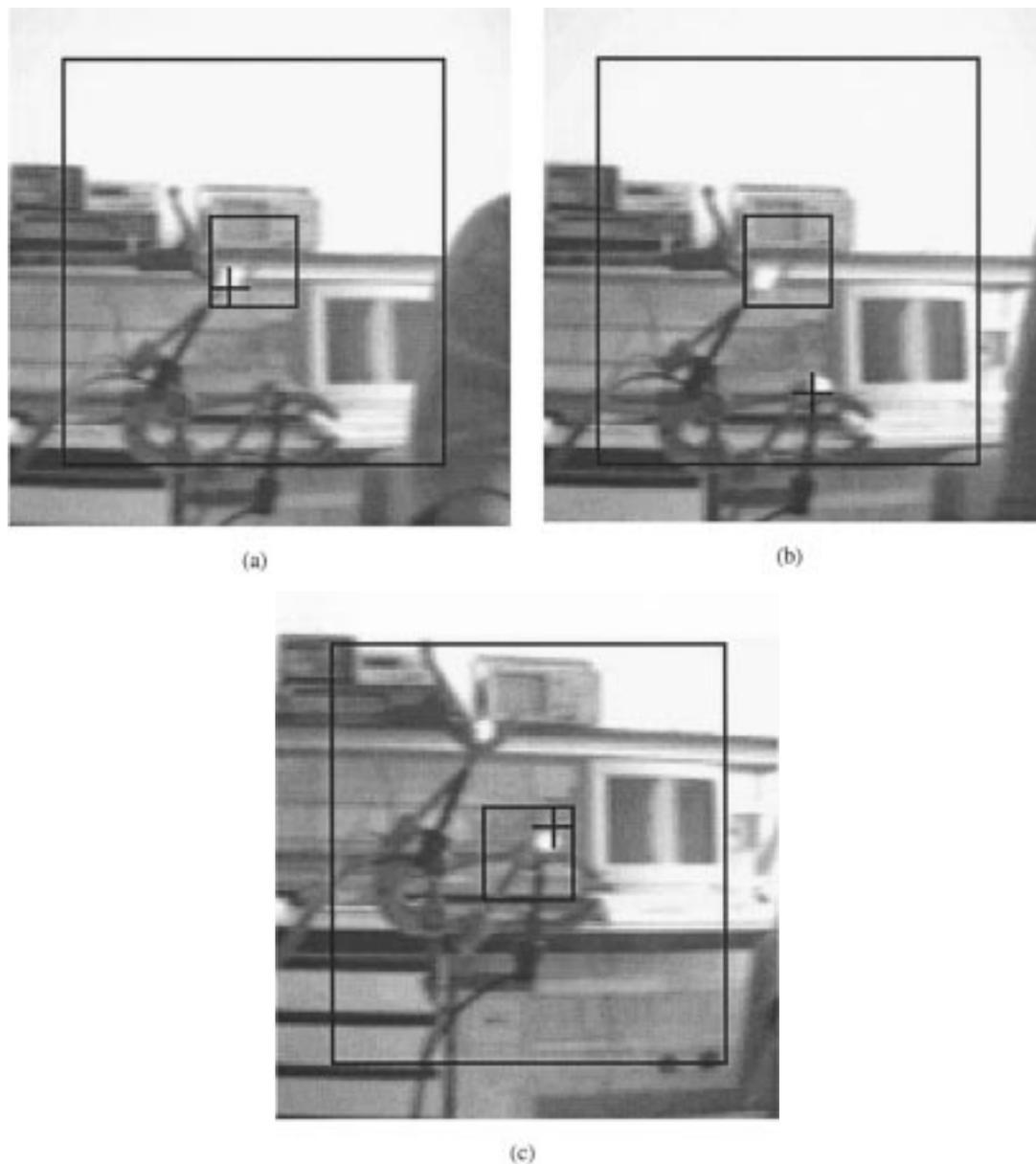
Fig. 9. Sequence of images showing the selection of a salient stimulus prior to and after a saccadic eye movement. (a) The system is attending the top LED, already centered on the central part of the imaging array. (b) The system selects the bottom LED, outside the central region of the imager. (c) The system performed a saccade toward the bottom LED, and is currently attending it.
