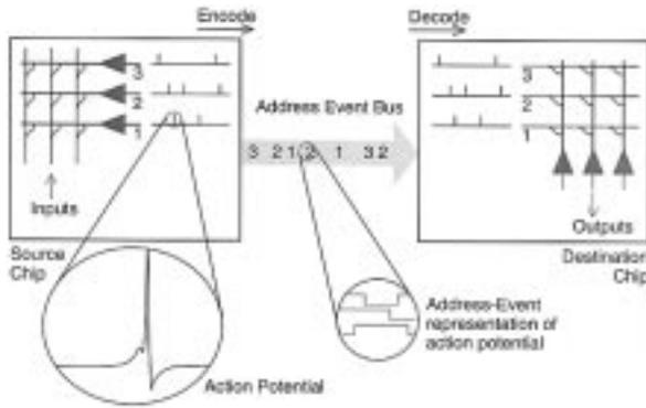
Fig. 3. Schematic diagram of an AER chip-to-chip communication example: “slow” action potentials generated by the “many” ( $N$ ) neurons of the source chip are transmitted as “fast” address events, on the “few” ( $\log N$ ) wires of the AE bus, to the synapses of the destination chip neurons.
