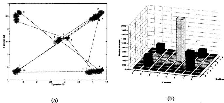
Figure 3: (a) Output of the position-to-voltage circuits of the selective attention architecture measured over a period of 300ms, in response to a test stimulus exciting four corners of the input array at a rate of 30Hz and a central pixel at a rate of 50Hz; (b) Histogram of the chip's output address-events, captured over a period of 13.42s in response to the same input stimulus.
