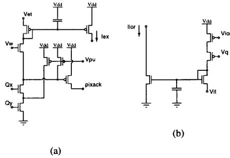
Figure 1: Synaptic circuits. (a) Input excitatory synapse; (b) Inhibitory synapse
