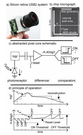
Fig. 2 Summarizes characteristics of Tmpdiff128 transient vision sensor. a) shows the vision sensor with its lens and USB2.0 interface; b) shows a die photograph labeled with the row and column from a pixel that generates an event with x,y,type output; c) shows an abstracted schematic of the pixel that responds with events to fixed-size changes of log intensity; d) illustrates how the ON and OFF events are internally represented and output in response to an input signal. Figure adapted from [1].
